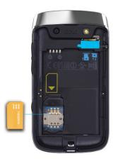
Slide the SIM card into the slot.
